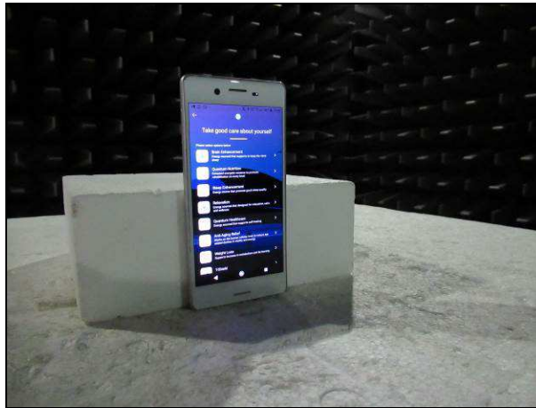
EN 55032 / CISPR 32: Radiated emissions device set-up
